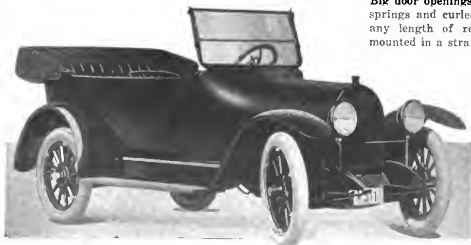
Five-passenger Kissel touring car with individual front seats and selling at $1,095. The motor is 3/4 by 5 in. and tires are 32 by 4
